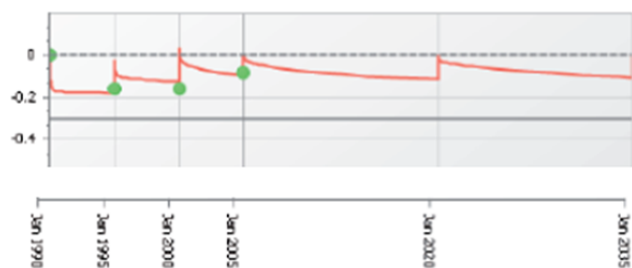
Figure 3. Predicted settlements and (green dots) predicted maintenance moments.
