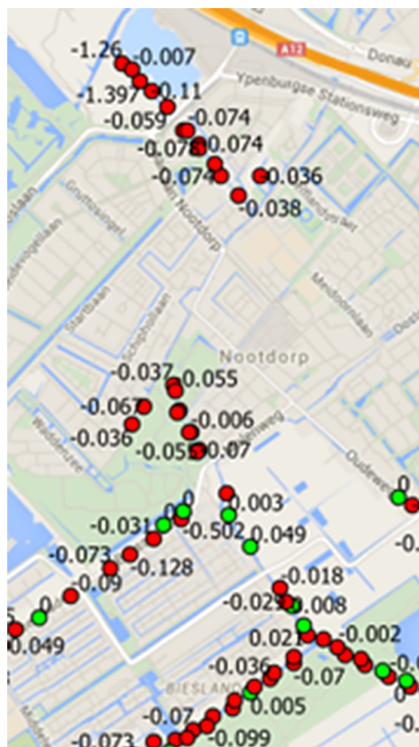
Figure 4. Calculated change in stability factor. Green dots mean an increase of the safety factor while the red ones indicate a decrease. The indicated values are the calculated decreases and increases.
