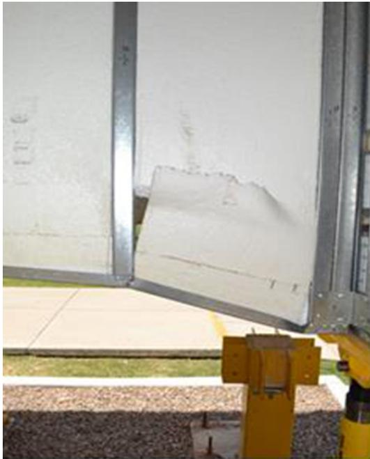
**Figure 4.** Excessive deformations in bottom track and fail of polystyrene.
